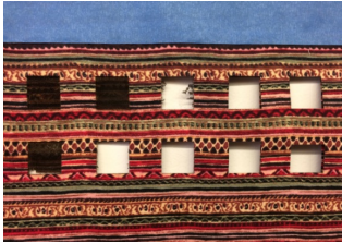
Figure 6: Testing power and speed on layered flannel fabric.
